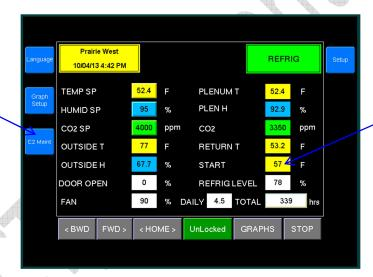
START; temperature OSA needs to equal for the system to begin Cooling Mode.
