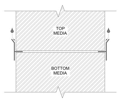
Vertical T-bars for vertical joints where media is inserted where a vertical gap could be present after installation. If a bank should be greater than 120" (3m) in height, then two separate systems need to be installed on top of each other. For the reasons above, two separate systems – top-supply and bottom-drain configurations – must be used.
