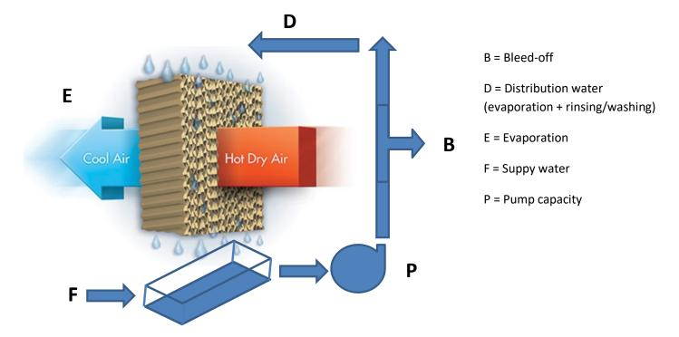
$$P(pump capacity) = D(distribution) + B(bleed-off)$$
