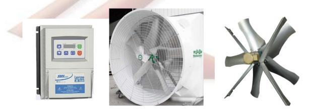
Notes: Fans include backdraft aluminum louver/shutter, extender cone for extra capacity and air throw. Can use 1 phase 208/230 VAC power while using variable speed drive – VFD converts 1 phase to 3 phase and allows automatic (via controller) or manual speed adjustment (via potentiometer or on keypad built into the VFD for speed adjustment), cone is attached on site. Motorized shutter available.
