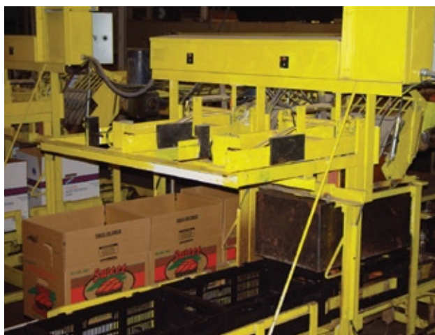
Figure 31. Automatic box fillers are integrated into electronic sizing equipment. (PHOTO BY G. HOLMES)
