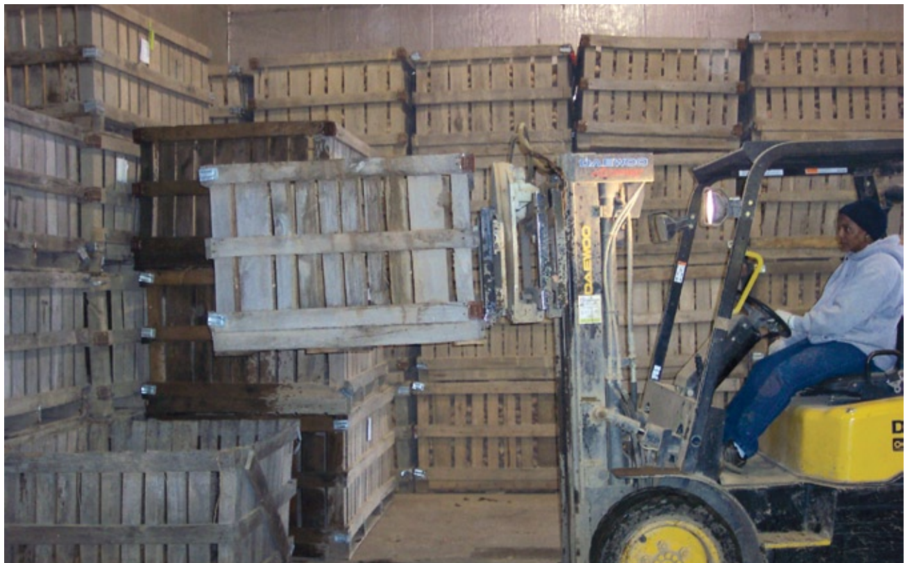
Figure 64. Extended forklift. (PHOTO BY T. SMITH)
