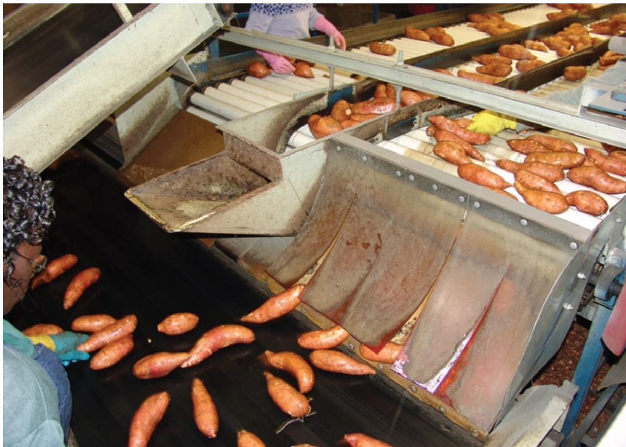
Figure 32. Install velocity-reducing flaps to slow root speed over packingline drops. (PHOTO BY G. HOLMES)
