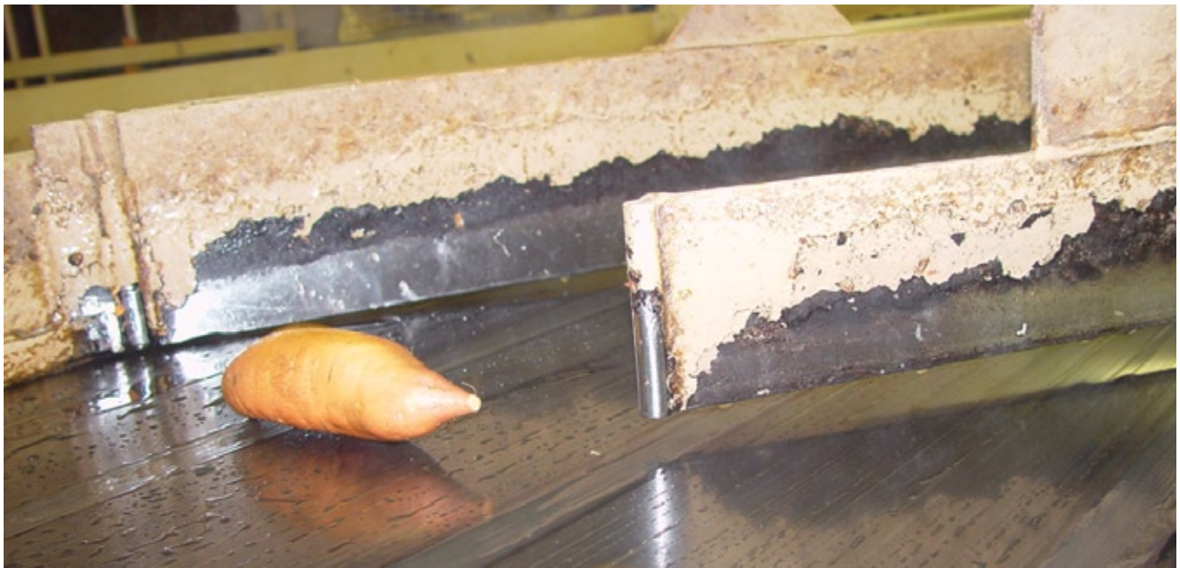
Figure 34. Packing line turn without padding. Note worn paint where roots make contact with metal guides. (PHOTO BY B. EDMUNDS)
