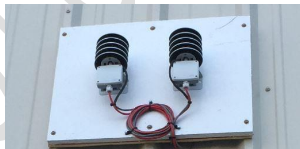
Outdoor temperature and humidity sensors with sun shields and insulated backboards
