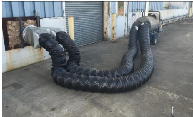
Heat exchanger with dual 12" heat resistant black PVC ducting 420,000 Btu/h Natural Gas
